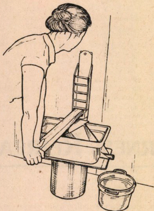
A Lever Press at Ramagiri Built by the Authors of Laurel's Kitchen
