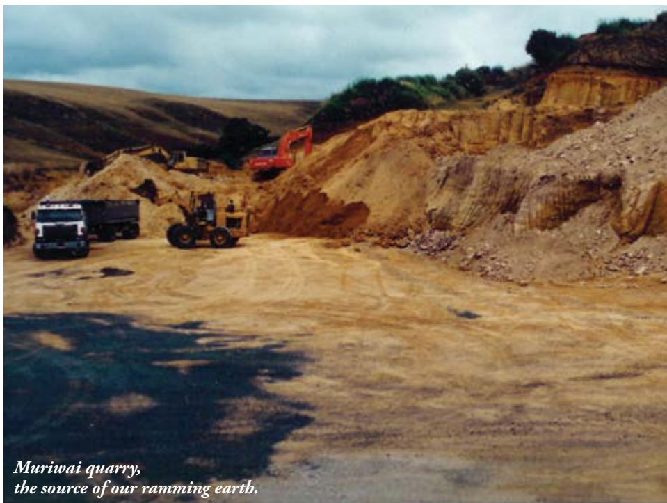
Freshly scraped face at Muriwai quarry showing natural variation in the ramming earth.
