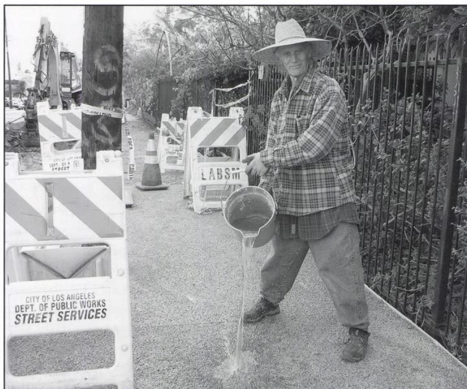
Perseverance pays: On the Shared Street Project, L.A. Eco-Villagers advocated for eco-savvy ideas like permeable sidewalks to help allow rainwater to replenish groundwater. Here, LAEV friend George Patton gives a demonstration.
