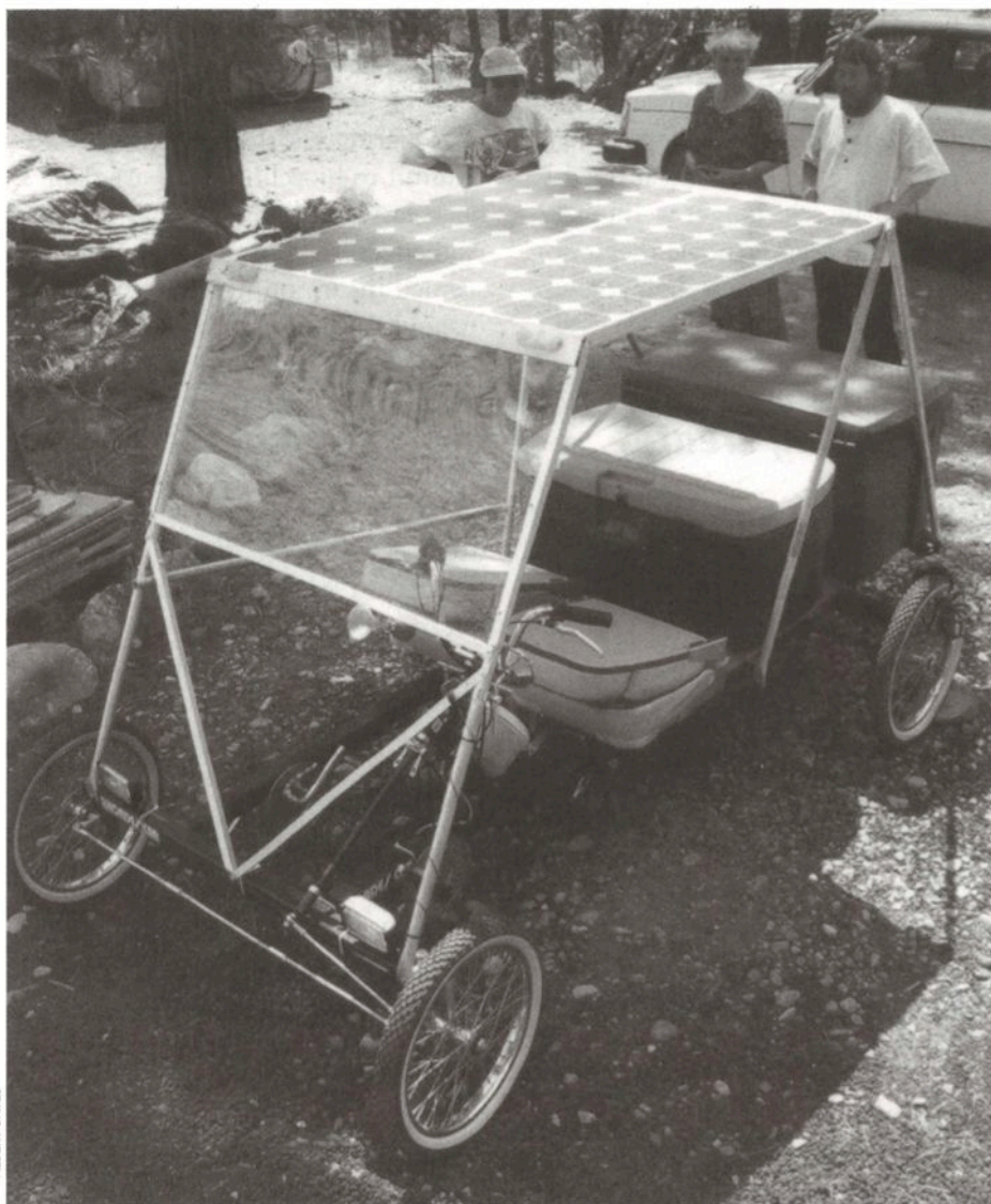
Solar and pedal power can be combined, like this pedal-assisted "solar car" from The Farm in Tennessee.
